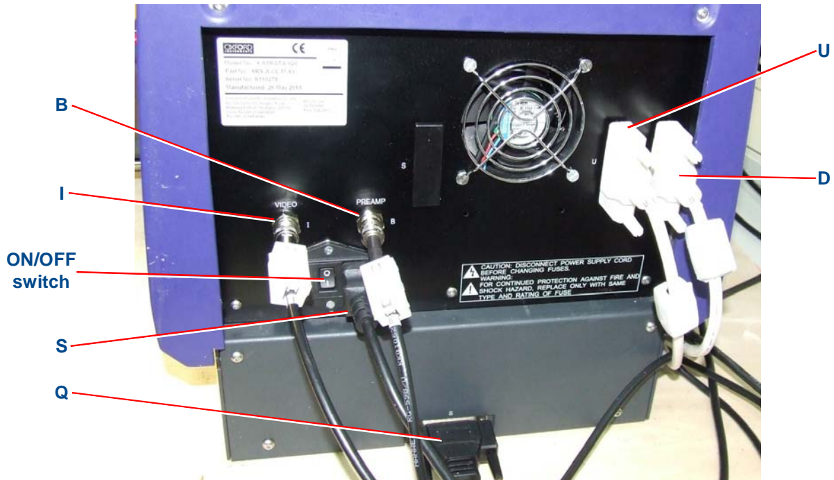
Fig. 3-1 Rear view of the X-Strata920
