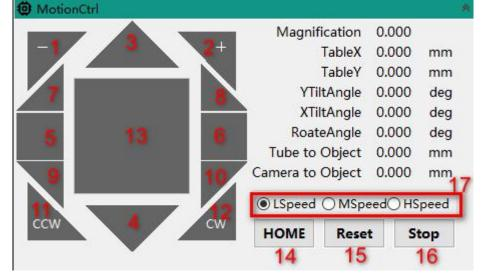
It is used to control the zero return of the equipment, the directional movement of each axis and the real-time display of the axis movement state after the movement.
