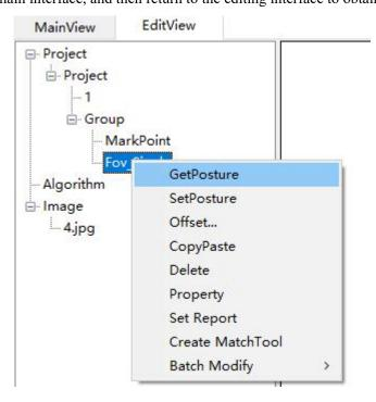
Only when the Fov obtains the posture, can the Tool be added to the current Fov posture picture, or you can select the Tool to be added in the toolbar, and drag the image with the mouse to generate the Tool.
