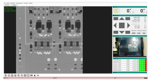
In the application software, the status bar is used to display the status of the system task being executed, the coordinate position of the mouse in the view area, and the movement status of the axis in real time.
