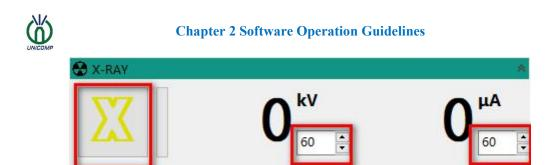
3. Under the X-Ray control module on the right control panel, turn on the X-ray and adjust the voltage and current.
