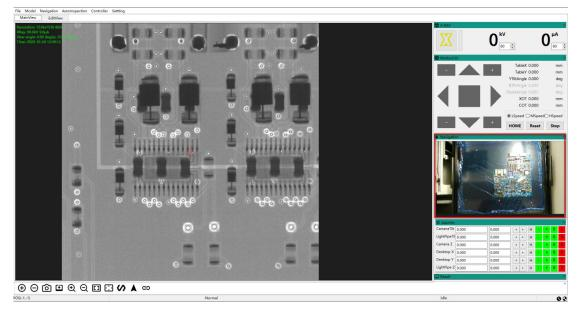
Navigation is used to quickly locate each part of the detected object according to the navigation map.
