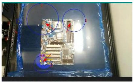
2.1. Calibrate the preset 3 calibration positions, find 3 calibration points in the main view, find point 1, alt+ right click in the main view, and adjust the movement to make the calibration position 1 at the center of the main view, click "calibration **Position 1**".
