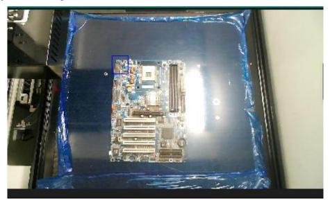
4. Under the navigation module on the right control panel, double-click the position of the detection object to move the navigation aperture to the specific position of the detection object or control the movement to the position of the detection object.
