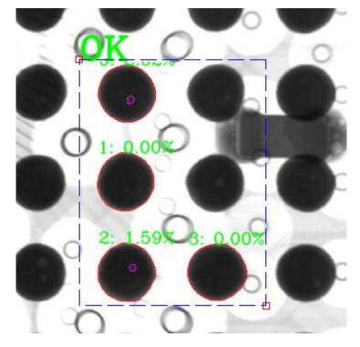
3. After selecting BGA, select the area to be detected on the image, as shown above.
