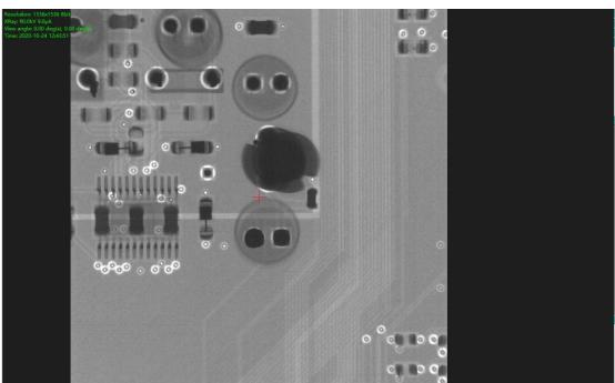
The image taken by the detected object is displayed, and the upper left corner displays the size of the current image, the voltage and current values used, the rotation angle of the camera/light tube, and the current time.
