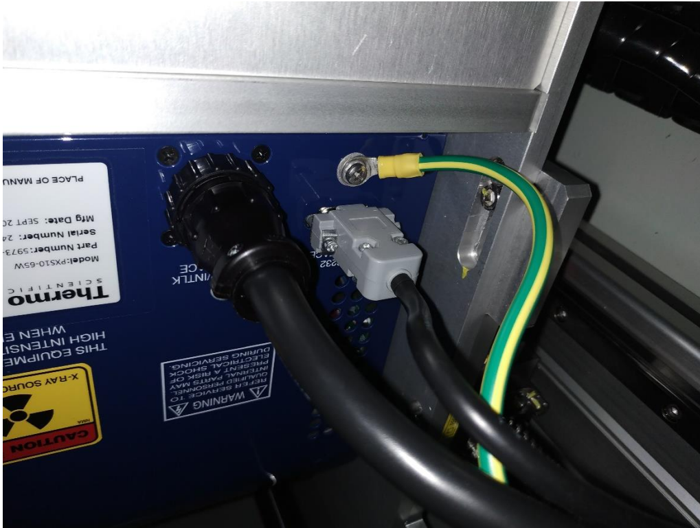
图 2.3.2-5 All cables of the X-Ray tube are connected
