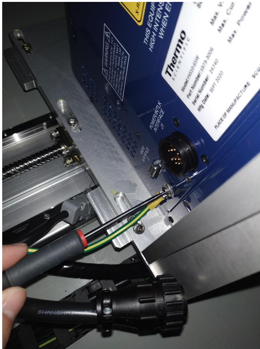
Figure 2.3.2-2 Connecting the ground wire
