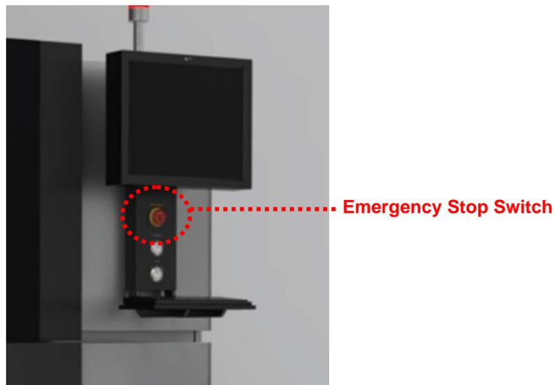
Figure 1-2 Emergency Stop Switch
